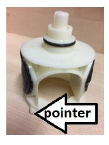
5. Fit the spring and plunger back into the diverter knob
