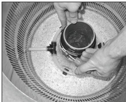
7. Tighten up the rubber connector to form a water tight seal.
