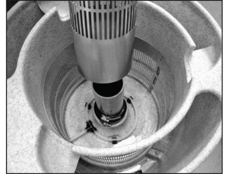
3. Loosen the upper clip on the rubber connector.
