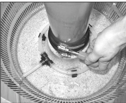
4. Invert the Pod and remove the 2 screws and plastic pipe support bracket.
